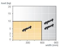
Mount 1 or 2 Titusoft mechanisms depending on drawer weight and width
